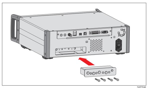
Figure 23. Manifold Installation
