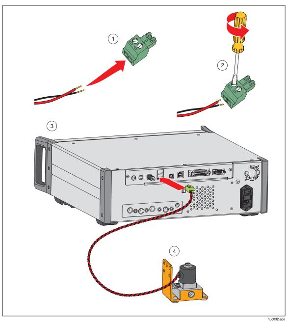
Figure 19. External Isolation Valve Connection
