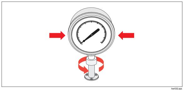
Figure 13. Tighten Gauge
