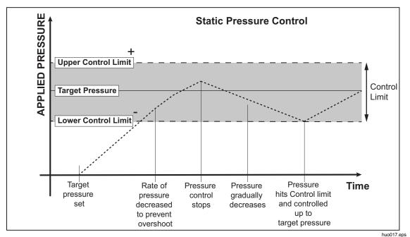
Figure 7. Static Pressure Control Mode Example
