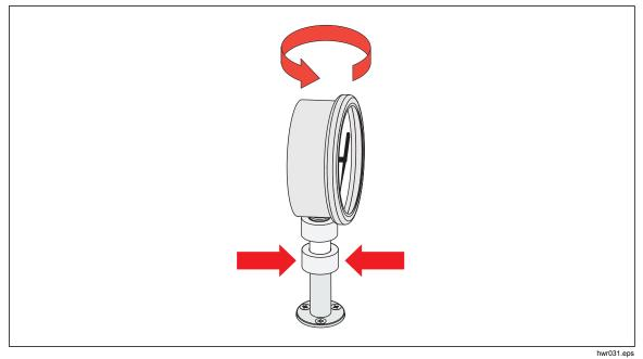
Figure 12. Adjust Gauge Position
