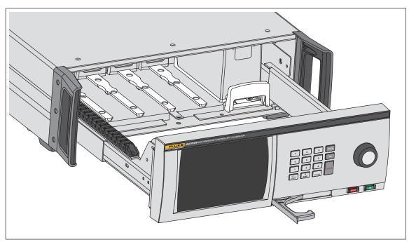
Figure 4. PCM Installation
