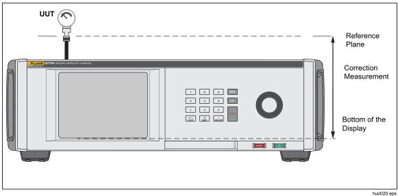
Figure 8. Head-Height Correction
