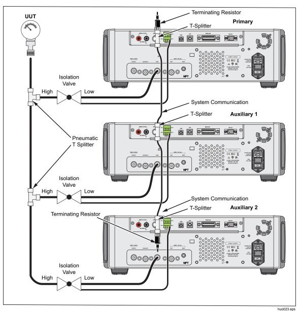
Figure 20. System Stacking Connections
