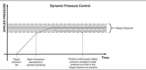
Figure 6. Dynamic Pressure Control Mode Example
