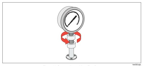
Figure 11. Connect Assembly to Test Port
