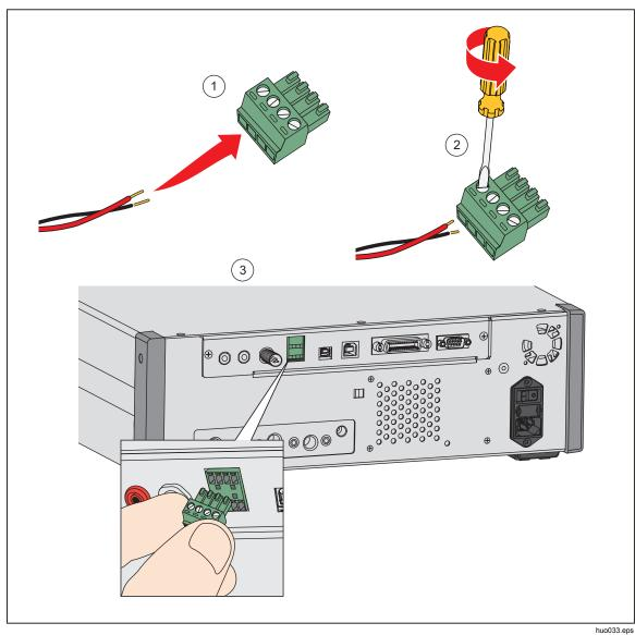
Figure 18. Driver Connections
