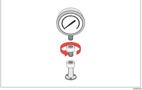
Figure 10. Screw on Gauge Adapter
