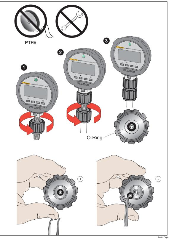
Figure 9. Replacing M20 O-ring
